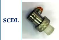
Single crystal delay line 0° compression wave probe with very good resolution for use on thin section material. Crystal diameter 6.3 mm. Replaceable delay line DL5. Maximum range in steel 18 mm. Fitted with Microdot connector as standard.
